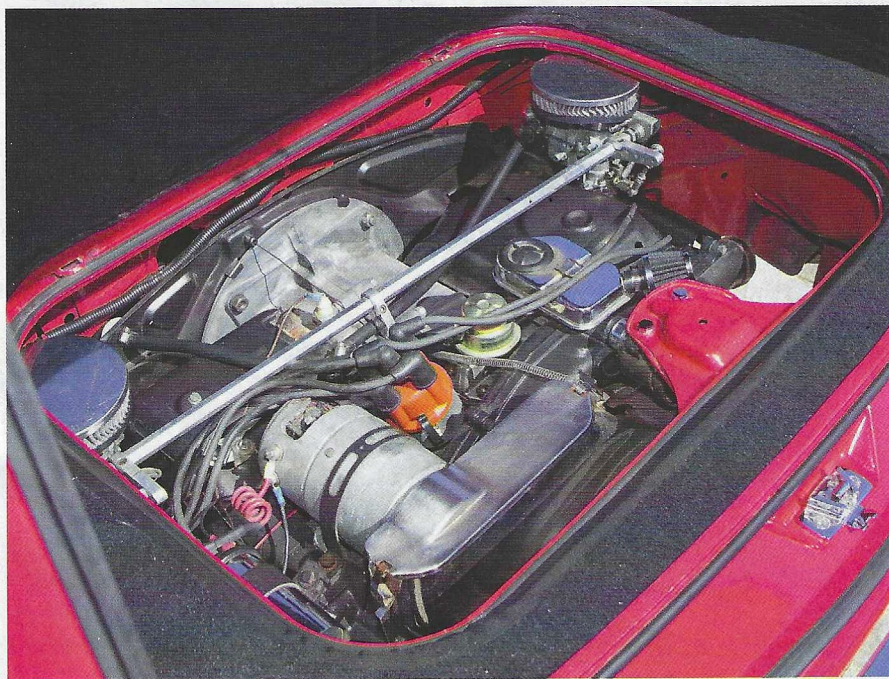
A stock Type 3 motor with dual EMPI carburetors is paired with a Freeway Flyer transmission to transfer power to the wheels. This combination has Paul cruising in comfort.
